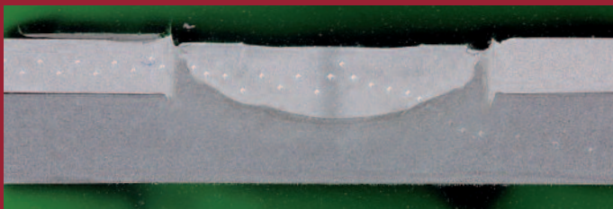
Makroschliff Al-Al Gussmaterial
